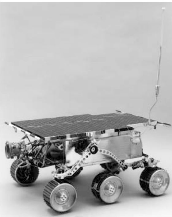
The Mars Pathfinder Rover contained three Light Weight Radioisotope Heater Units (LWRHUs).
