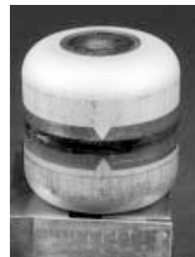
A General Purpose Heat Source (GPHS) fueled clad.
